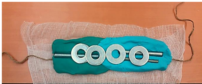
Fig. 4.9. Components' distribution in the forearm simulator.
