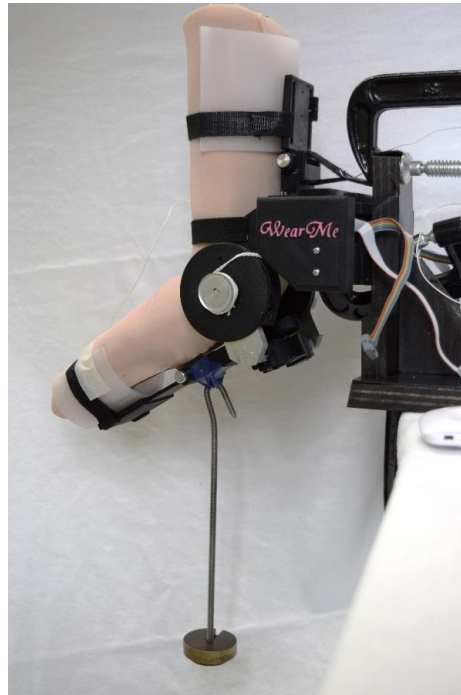
Fig. 4.8. The setup for the assessment of the mechanical stoppers. Photo credits: Hilary Luo.
